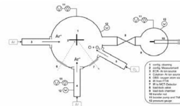
**Figure 1:** Schematic top view of the ion beam reactor.
