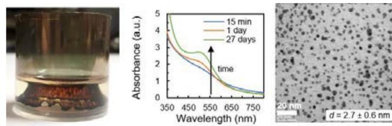
**Fig 1.** UV-VIS and TEM characterization of Au-NPs obtained by sputtering Au on castor oil.
