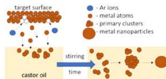
**Fig 2.** Scenario of Au-NPs formation in castor oil.
