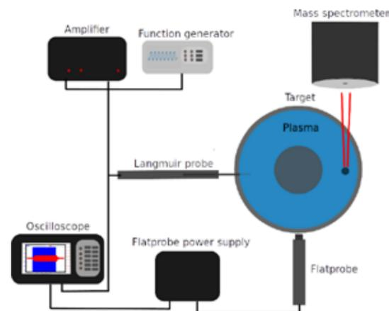
**Fig 1.** Schematic depiction of the experimental setup.
