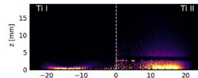
**Fig 1.** – Abel inverted false color image of titanium neutral emission (left) and titanium ion emission (right) at the end of a HiPIMS pulse. Titanium neutral emission is only observed close to the target because of neutral depletion by strong ionization.
