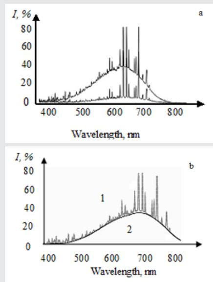
Fig.1. a – Typical emission spectra at different discharge power; b – Extraction of the thermal radiation spectrum (1 - initial spectrum, 2 – extracted spectra of thermal radiation).
