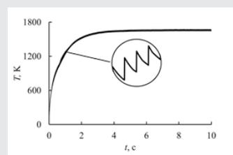
Fig. 2: Dependence of maximum temperature of titanium target of time (duration 250  $\mu$ s, frequency 100 Hz); also additionally were shown pulsations between high-power pulses.
