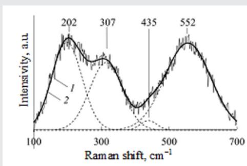
Fig. 2. Raman spectra of the sample 2 (fig. 1) and the result of the simulation: 1 – the measured spectrum; 2 – model
