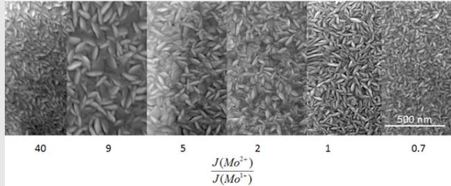
SEM micrograph of the film morphology as a function of the ion flux ratio of Mo<sup>2+</sup> and Mo<sup>1+</sup>.
