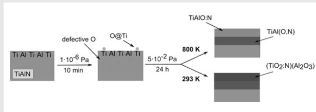
**Figure 1: Surface oxide structure during different stages of the thermal oxidation of Ti<sub>0.5</sub>Al<sub>0.5</sub>N.**
