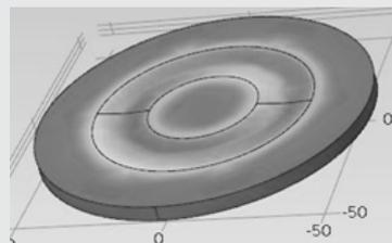
Fig. 1: The result of simulation of impact of pulses on titanium target on the tenth second (duration 250  $\mu$ s, frequency 100 Hz).
