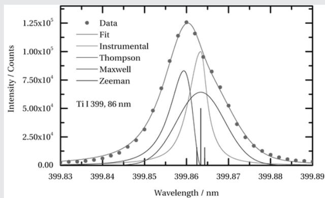
**Fig. 1: Measured and fitted Titanium neutral emission line with individual components of the fit function**
