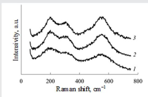
Fig. 1. Raman spectra of films TiN, deposited at current density 32  $\text{mA}/\text{cm}^2$  and flow of  $\text{N}_2$  (sccm): 1 – 2; 2 – 4; 3 – 6;
