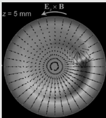
**Figure:** Plasma potential measured for the case of one dcMS spoke, red: positive and blue: negative, with the largest difference about 80 V, for more details see [4].
