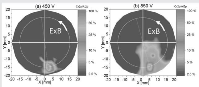
Fig. 1: Chromium concentration map for the low power case (a) and the high power case (b)
