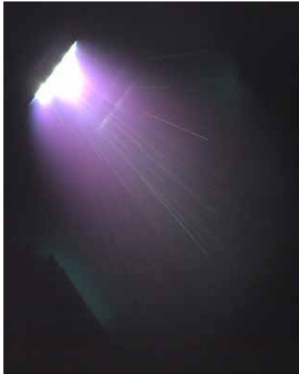
Fig: A Laser-arc discharge with macroparticles
