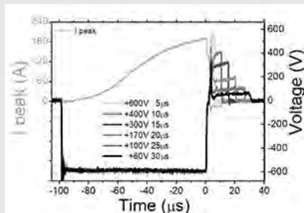
Figure. Discharge peak current and voltage waveforms for different voltage reversal configurations (ranging from +70 to +600V and from 5 $\mu$ s to 30 $\mu$ s)
