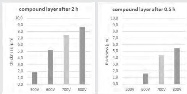
Figure 1: Development of compound layer thickness with increasing voltage for short time plasma nitriding processes, 2 hours on the left and 0.5 hours on the right constant parameters: pressure 300 Pa; temperature 565°C; pulse-to-pause ratio 100 µs: 400 µs; atmosphere 80% nitrogen, 20% hydrogen
