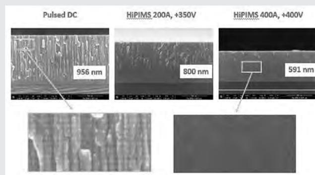
Figure. SEM images of TiO<sub>x</sub> layers deposited onto Silicon at RT by both Dc-Pulsed and HiPIMS with voltage reversal.
