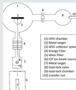
We present first results and outline the potential of the ion beam experiment. We show iSEECs in dependence of the ion energy of commonly used HiPIMS target materials (Al, Ti, Cu).
