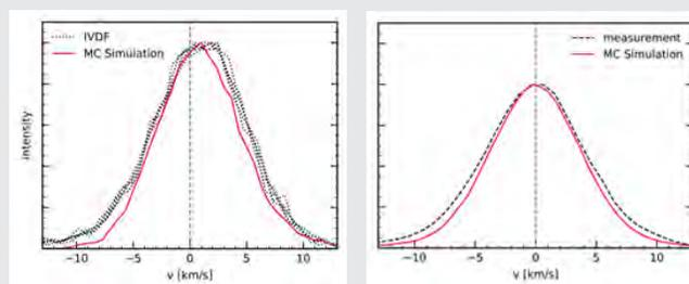
Fig.1 Measured velocity distribution function of titanium ions (IVDF) and the VDF obtained from the model in the direction perpendicular to the target surface.
